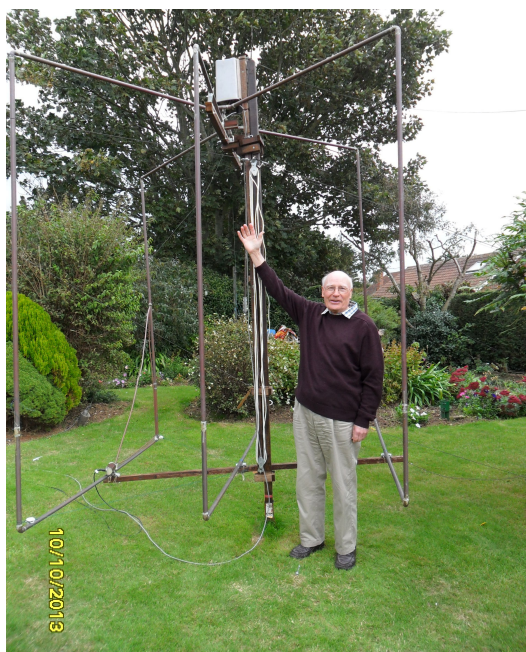
Illustration 4: Antenna telescoped down for maintenance
