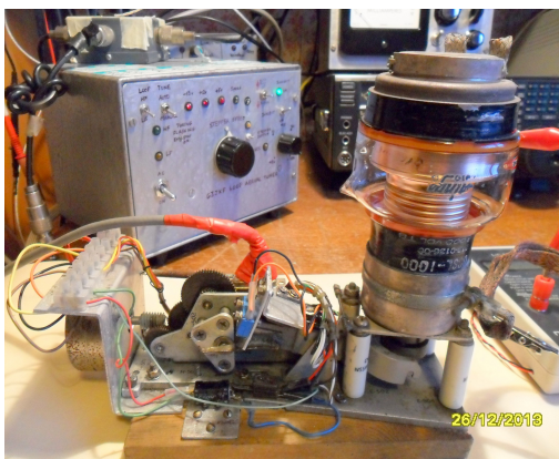
Illustration 6: Vacuum Capacitor from Collins 180L with modified motor and pinion.
