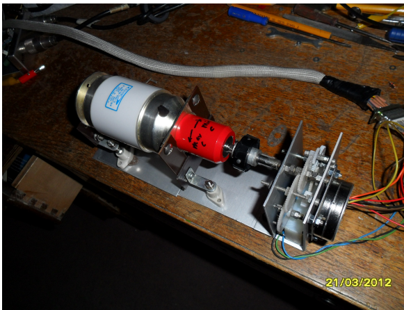
Illustration 8: Vacuum Capacitor Assembly with homebrew gearbox and stepper motor.
