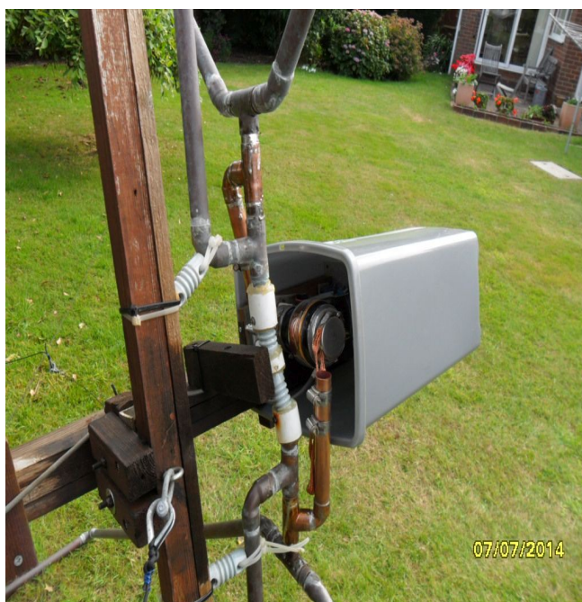
Illustration 5: View of Vacuum Capacitor connections to LF Triple Loop Antenna
