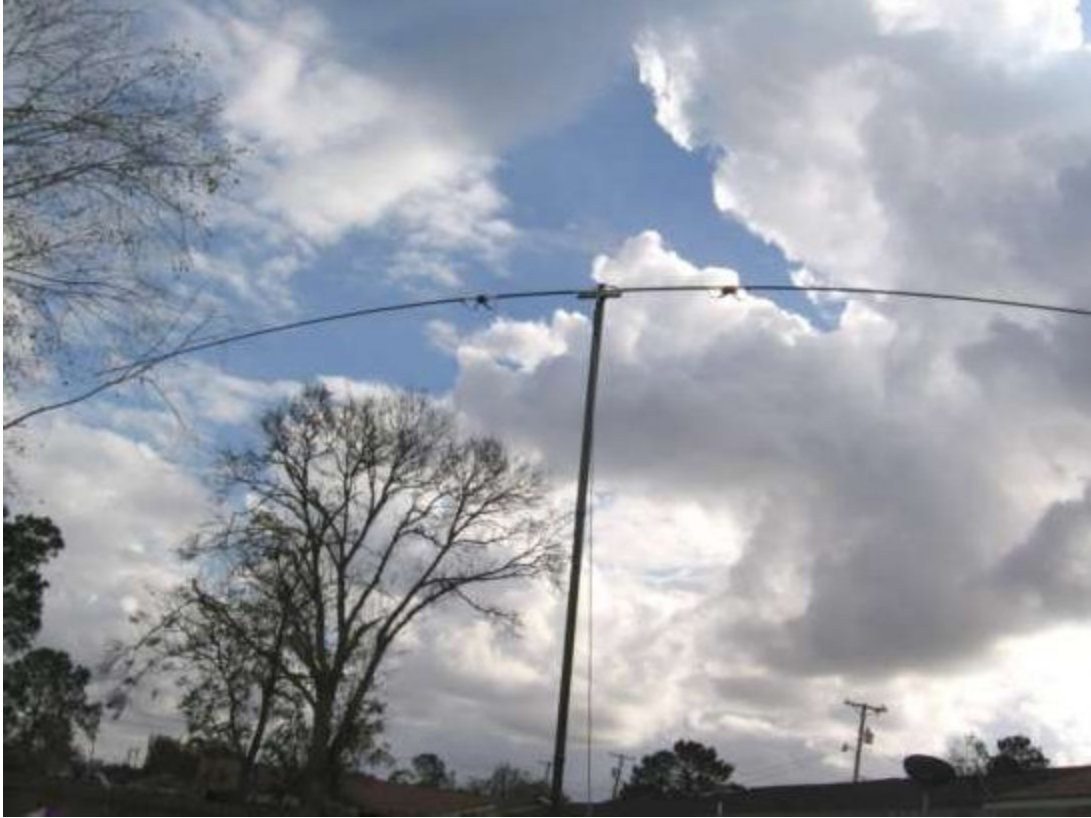
28 It's up, 40 meter coils in use, and the whip ends adjusted for best SWR.
