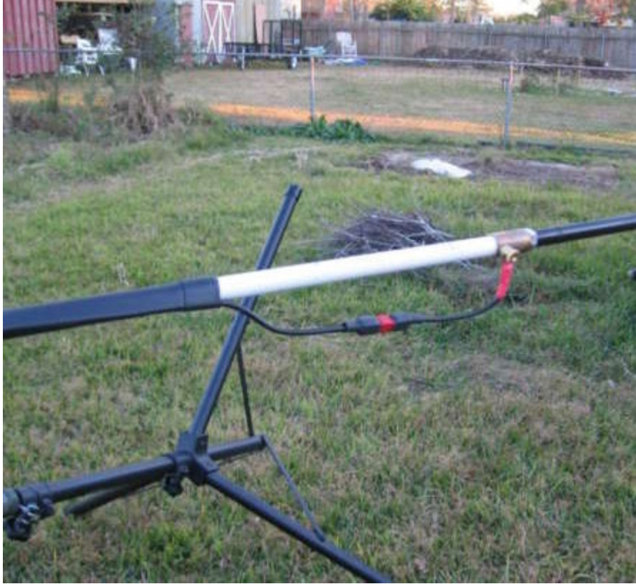
17 Whips screwed on.jpg -- Screwed on and fully extended. The dipole is about 12' on each side.
