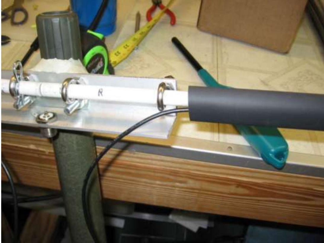
11 Heat Shrink Arms a.jpg — 3/4" heat shrink is slipped over the fiberglass arms and wire, to about 1" from the end of the aluminum angle center support.
