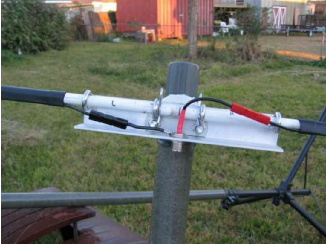
16 Center wired.jpg — You can see here how I finished the center and connected to the arms with Power Poles. As you can see, we are now outside... somethings gonna happen!
