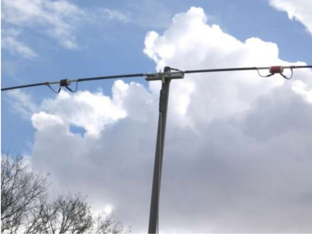
29 Closeup. The coils are just slipped over the ends, and the jumpers hooked to the coils. Anderson Power Poles used here, too.
