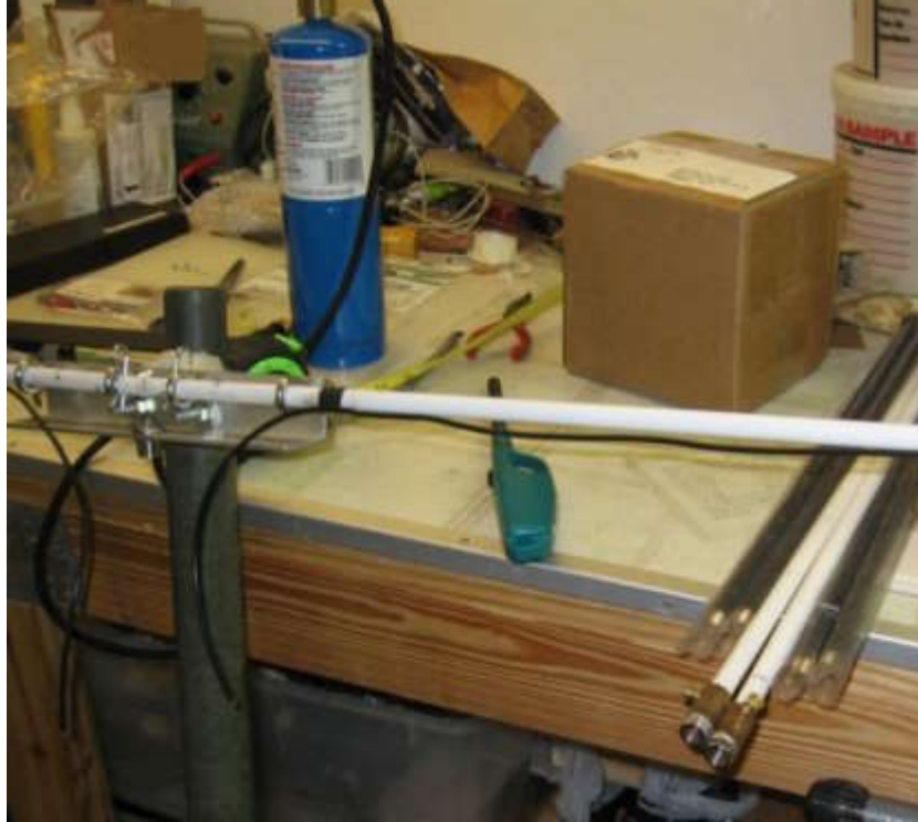
10 Wiring Arms.jpg — Here some 14 gauge insulated wire is held in place with some short pieces of 3/4 heat shrink, shrunk in place. This 14 ga wire will be the middle part of the dipole.
